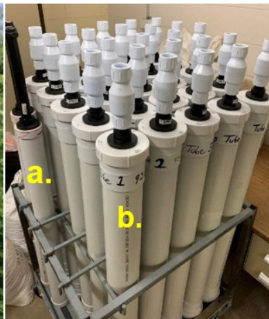
Figure 2. PVC silage compacting device (a.) and ensiling tube (b.)
